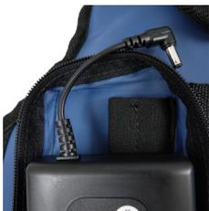
Open battery compartment and disconnect battery as shown, leave disconnected sixty (60) seconds
