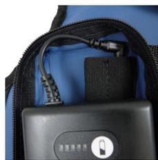
Plug battery back in, controller should beep twice when plugged back into battery
