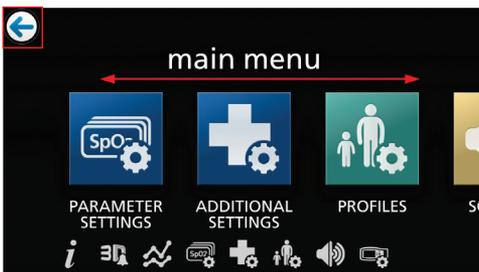
Icons at the bottom edge of the displayed menu screen correspond to the settings. Touch an icon to jump to the setting on the displayed menu screen.
