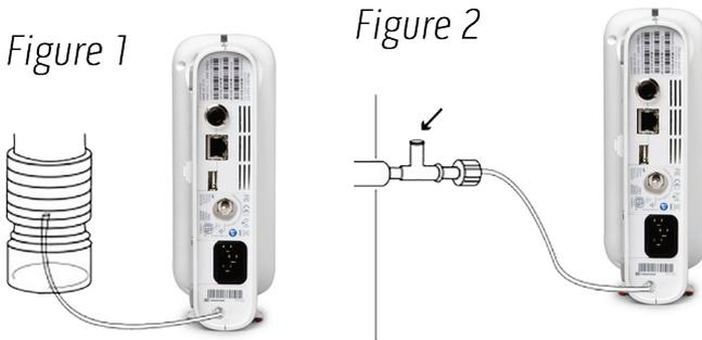
Two different ways of scavenging the exhaust gas; through a ventilator reservoir (Figure 1) and directly to a scavenging system (Figure 2). In both cases, generate a deliberate leakage to avoid vacuum in the ISA's exhaust gas tube.
