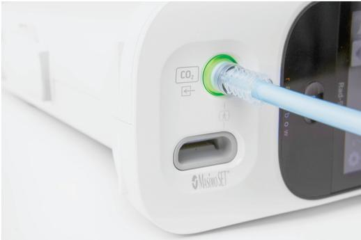
3. Breathe briefly into the sampling line and check that a valid CO<sub>2</sub> waveform and values are displayed.
