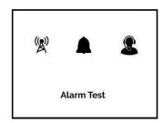
The system will begin by testing the High Priority Alarm. The High Priority Alarm consists of a 10-beep sequence separated by 2.5 seconds of silence and the LCD screen flashes red. The alarm symbol will appear on the screen.
