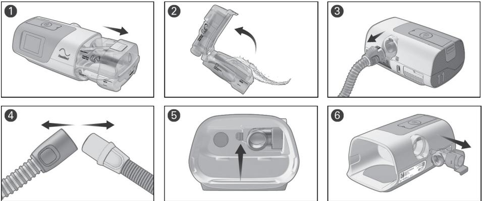
1. Hold the humidifier tub at the top and bottom, press it gently and pull it away from the device.
