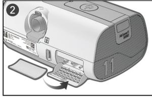
1. Open the air filter cover and remove the old air filter. The air filter is not washable or reusable.
